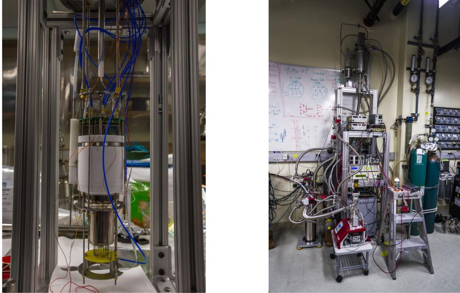
Figure 4: (Left) Fully assembled LAr TPC at UCLA. (Right) TPC installed within cryostat and integrated into full cryogenics, high voltage, and data acquisition systems.
