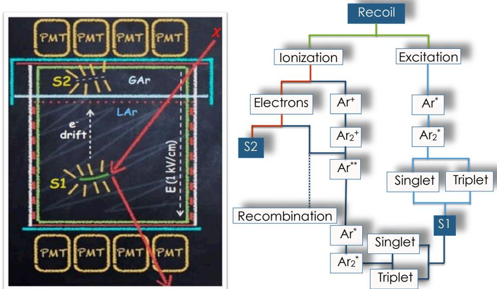
Figure 1: (Left) Schematic of a LAr TPC. (Right) Scheme for the ionization and scintillation branches.
