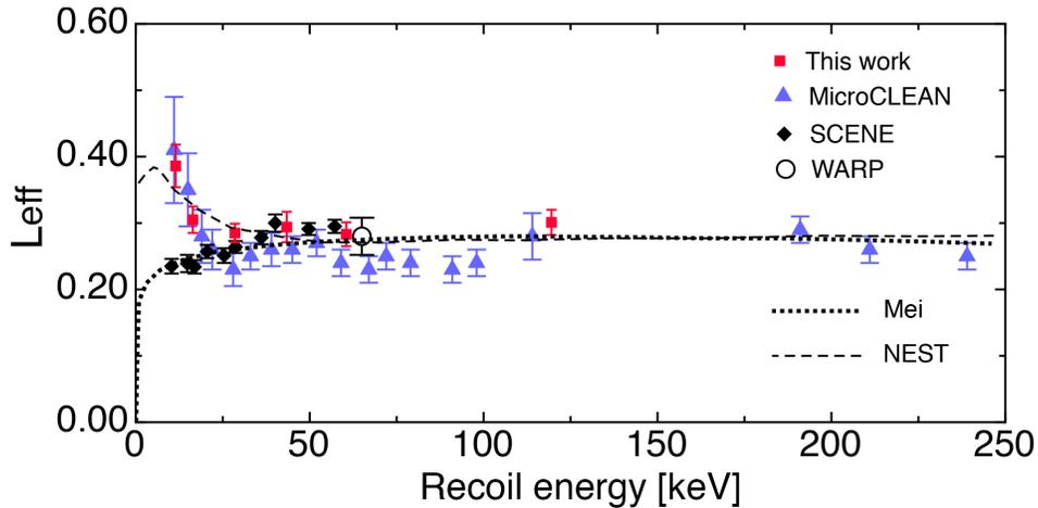
Figure 2: Previous measurements of relative scintillation efficiency ( $\mathcal{L}_{\text{eff}}$ ) in other experiments. Red squares (“This work”) refer to Ref. [8].
