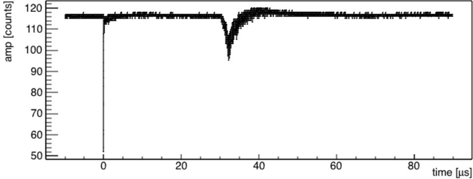
Figure 5: Example event showing the S1 and S2 signals.
